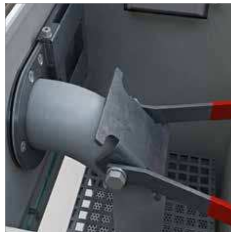
Safety flap prevents vacuuming without liquid container
