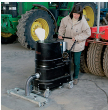
R01 R022 explosive dust with floor vacuuming device in the agricultural industry
