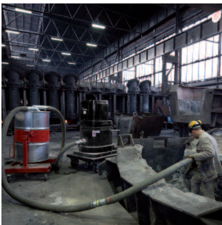
DS 2520 with pre-separator in steel production
